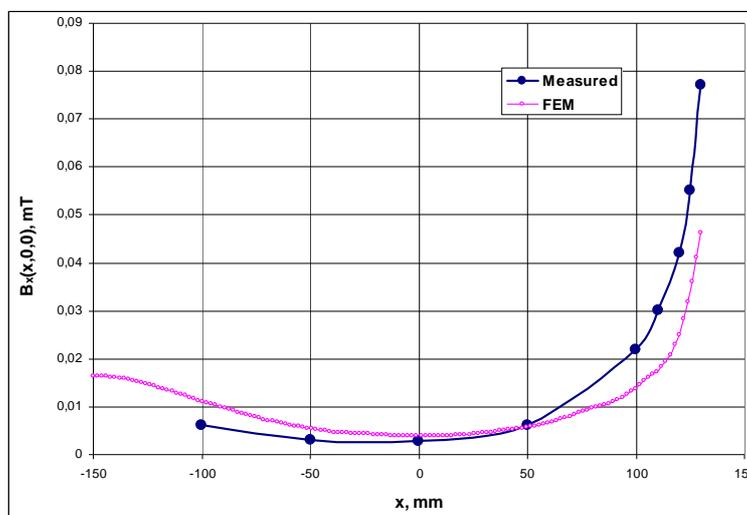
*Fig. 4: Measured and simulated axial magnetic field  $B_x(x)$  along the symmetry axis of a circular MUMETALL® cylinder with lids at both ends, aligned coaxially in the centre ( $x = 0$ ) of a Helmholtz coil system. The lines between the dots are guides for the eye only.*
