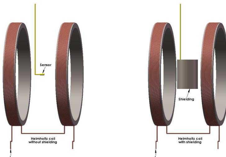
*Fig. 1: Sketch of the Helmholtz coil system without (left) and with (right) the magnetic shielding under test.*
