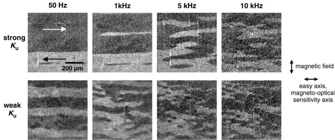
Fig. 5. Domain refinement with increasing frequency of nanocrystalline cores with strong and weak  $K_u$ . Arrows indicate the magnetization direction.
