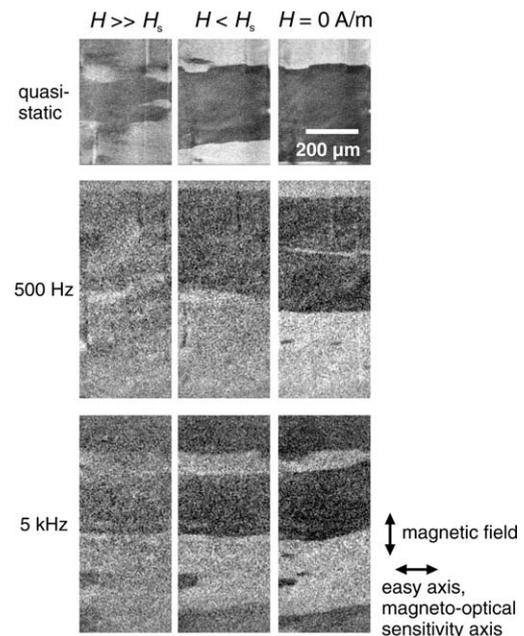
Fig. 7. Magnetization process of the core with strong  $K_u$  in a decreasing magnetic field for quasi-static remagnetization, at 500 Hz and at 5 kHz. Homogeneous rotation dominates the magnetization process. Slight wall displacements are also visible.
