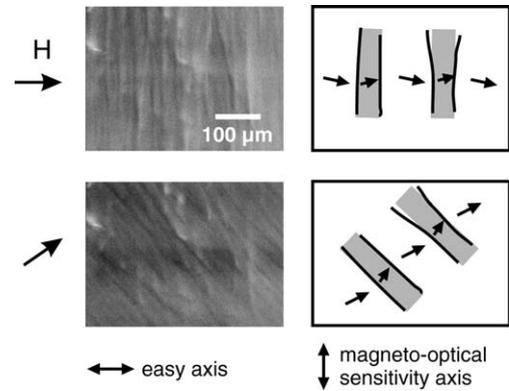
Fig. 9. Domain images and corresponding sketches of the stripe-like domains at an applied field of 20 kA/m in different directions. The domains are aligned perpendicular to the applied field.
