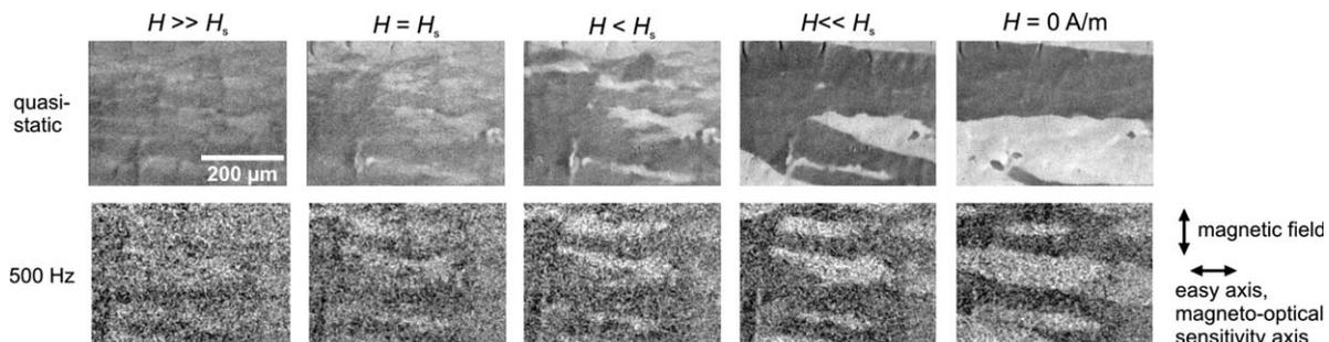
Fig. 8. Magnetization process of the core with weak  $K_u$  in a decreasing magnetic field for the quasi-static case and at 500 Hz. The wide domains arise at stripe-like residual domains that persist far beyond the “technical” saturation field  $H_s$ .
