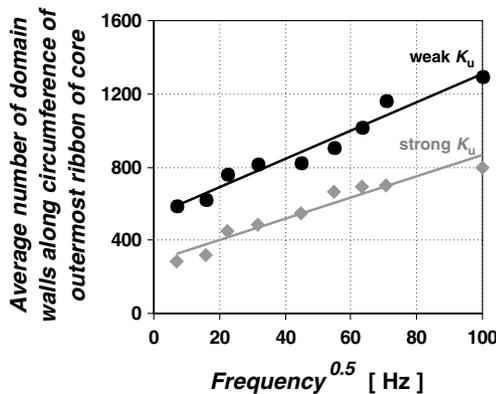
Fig. 6. Average number of surface domain walls along core circumference vs. square root of the frequency.
