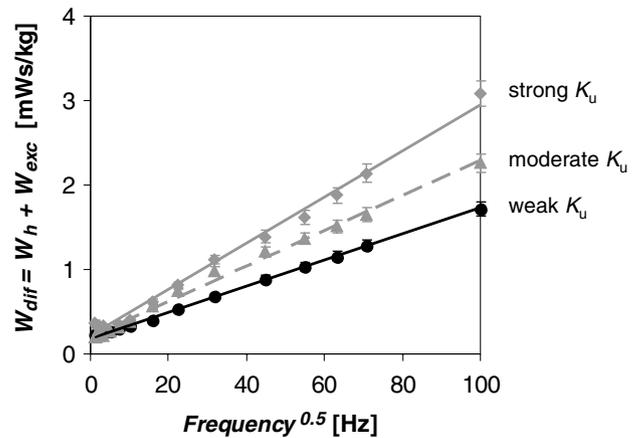
Fig. 4. Sum  $W_{\text{dif}}$  of hysteresis loss  $W_h$  and excess loss per cycle  $W_{\text{exc}}$  vs. square root of frequency deviates from the typical linear behavior only at low frequencies.
