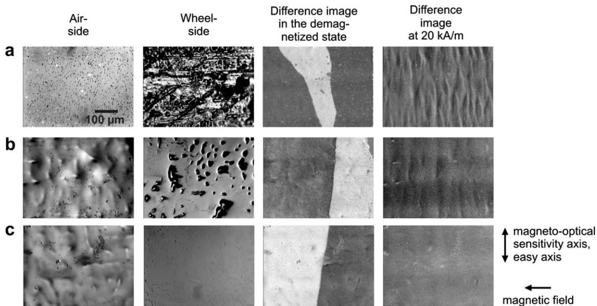
Fig. 10. Appearance of stripe-like domains in the difference image at high field strengths depends on the roughness of the wheel-side. The difference images are obtained at the indicated spot of the air-side: (a) unpolished wheel-side, polished air-side; (b) slightly polished wheel-side, unpolished air-side; and (c) strong polished wheel-side, unpolished air-side.
