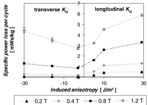
Fig. 1. Specific power loss per cycle at a frequency of  $10\ \text{kHz}$  and various peak induction levels ( $0.2$ – $1.2\ \text{T}$ ) for nanocrystalline tape wound cores with different strengths of field-induced anisotropy  $K_u$ . Negative values of the induced anisotropy mark transverse  $K_u$ , positive values longitudinal  $K_u$ .
