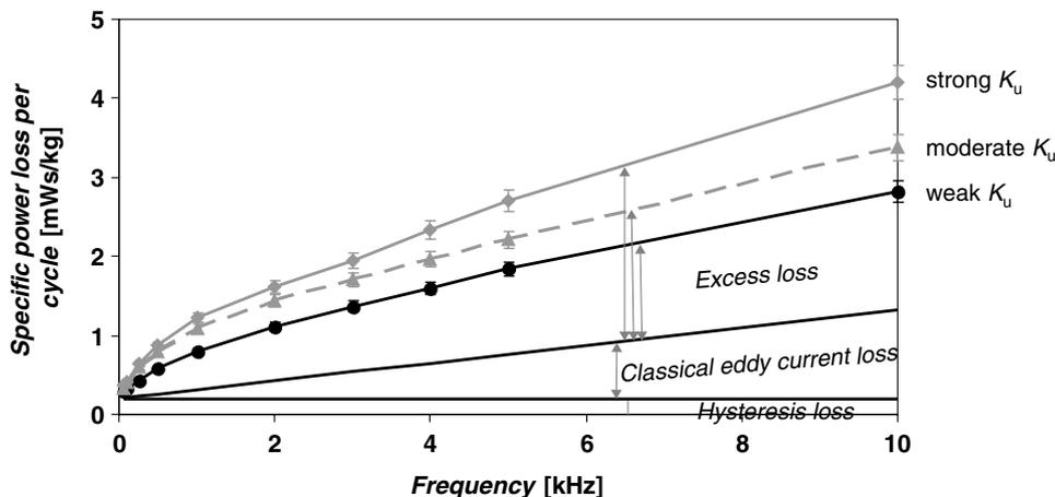
Fig. 3. Specific power loss per cycle vs. frequency. The excess loss component increases with increasing  $K_u$ .
