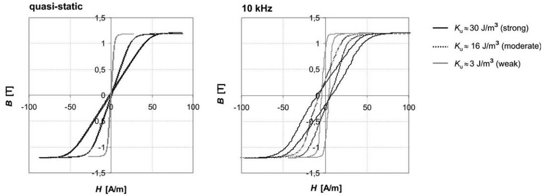
Fig. 2. Hysteresis loops of three nanocrystalline tape wound cores with different strengths of transverse field-induced anisotropy  $K_u$  at very low frequencies (left) and at 10 kHz (right).
