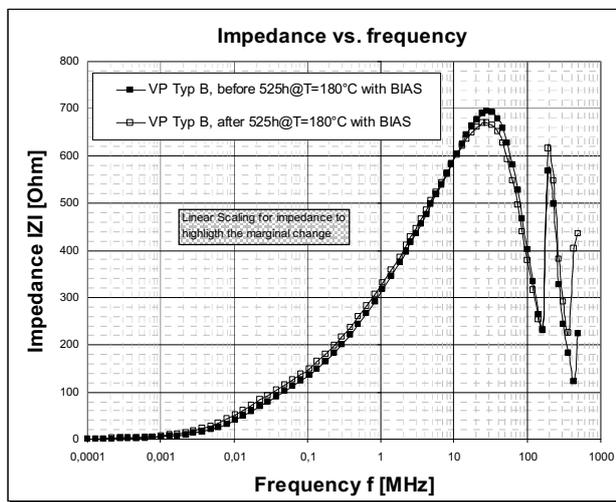
Figure 10: Impedance versus frequency for the Common Mode Choke (Typ B; semi- finished version ) welded in the final powerframe before and after temperature storage test at  $T=180^{\circ}\text{C}$  for  $t=525\text{h}$  under unbalanced conditions.
