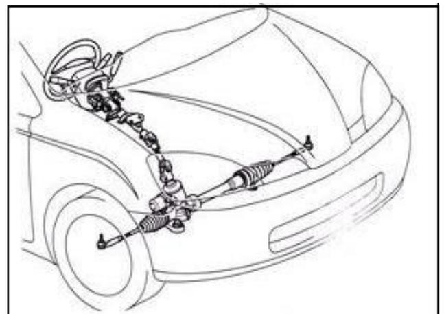
Figure 1: Schematic drawing of an Electronic Power Steering system (pinion gear version). Further information about the diversity of EPS-systems is given in [1].
