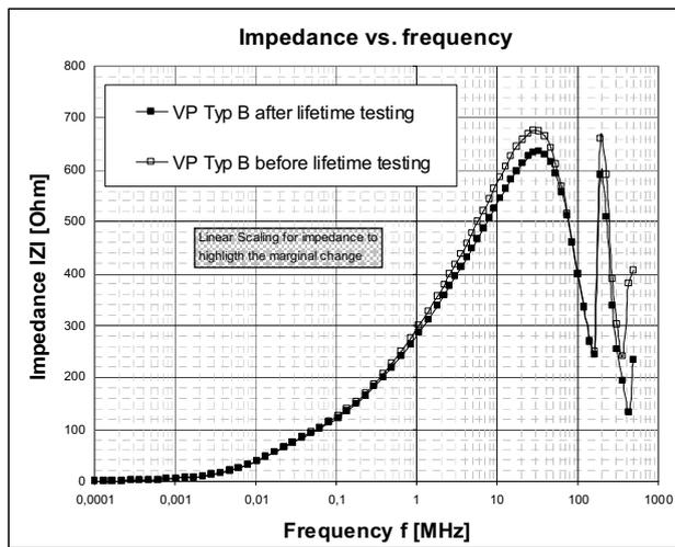
Figure 11: Impedance versus frequency for the Common Mode Choke (Typ B; semi- finished version ) welded in the final powerframe before and after lifetime test.
