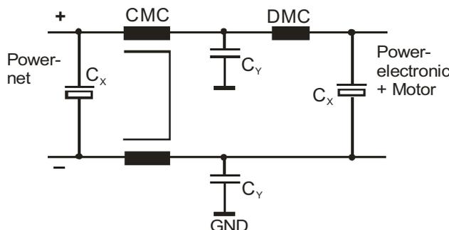
Figure 3: Typical EMI-filter for EPS-systems
