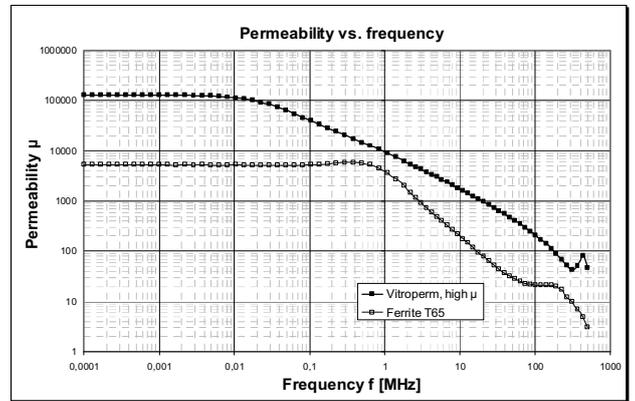
Figure 8: Permeability  $\mu$  versus frequency  $f$
