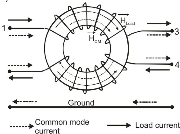
Figure 2: Principal function of a Common Mode Choke
