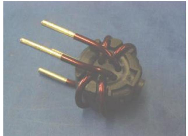
Figure 4: Common Mode Choke for EPS-systems (Type A; Version with thick wire  $d=2,24\text{mm}$ ),  $I=25\text{A}$ ,  $I_{\text{max}}=120\text{A}$  for  $t=2\text{sec}$ .
