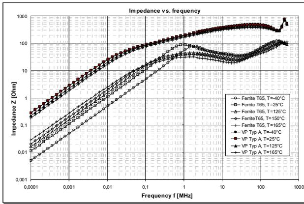
Figure 6: Typical impedance versus frequency behaviour for Type A (wound version, see figure 4) in comparison to a standard EMI-ferrite with a similar component size. Temperature range  $T=-40^{\circ}\text{C}$  to  $+165^{\circ}\text{C}$ .
