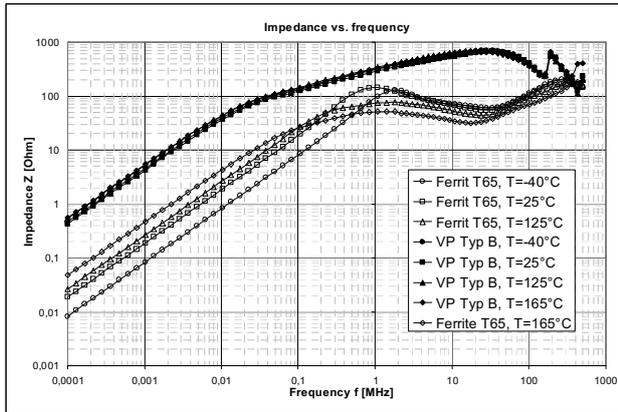
Figure 7: Typical impedance versus frequency behaviour for Type B (see figure 3) in comparison to a standard high temperature EMI-ferrite of the same component size. Temperature range  $T=-40^{\circ}\text{C}$  to  $165^{\circ}\text{C}$ .
